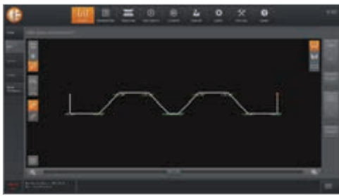
■ 2D part drawing can be made on the control screen
