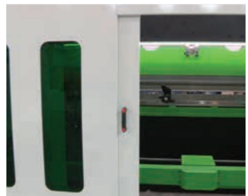
■ Maximize your safety with the rear sliding cover and switch. Check inside the machine by means of the windows (S)
