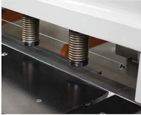
■ Shadow line generates projection over sheet metal to be cut to provide high quality and precise cutting (S)
