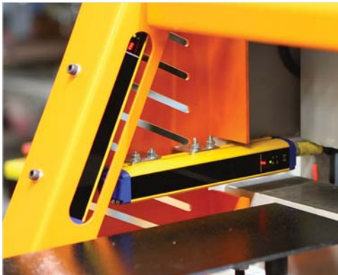
■ Illuminated finger protection system with high safety protection degree and enabling fast operation (O)
