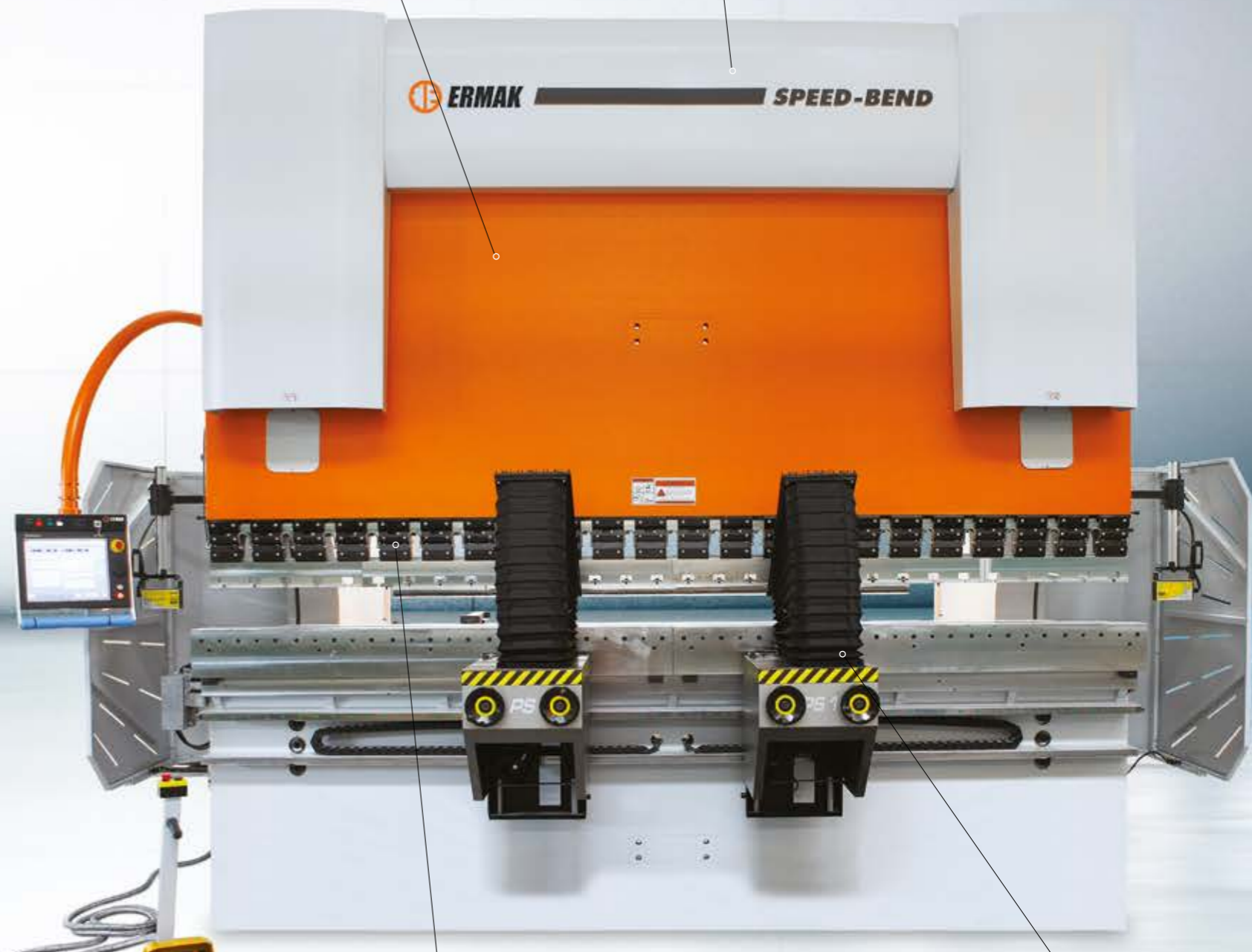
Top clamping promecam Promecam type top clampings can easily be put on and off.
