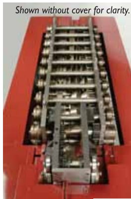
Optional Pivoting Head Quad Cutter Attachment (24 gauge max.) for slitting blanks for "S" and Drive Cleats. Cutter-head disengages for running pre-cut blanks.
