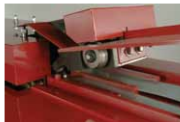
Optional Pivoting Head Quad Cutter Attachment (24 gauge max.) for slitting blanks for "S" and Drive Cleats. Cutter-head disengages for running pre-cut blanks.
