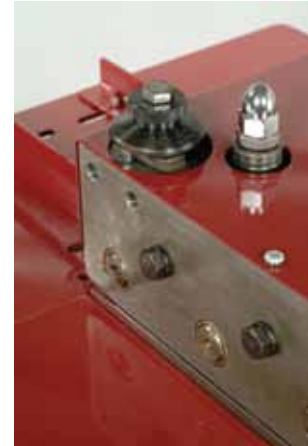
Exclusive dial adjustment for instant changing for all gauges 20-30.
