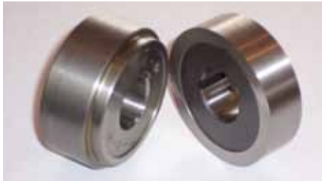
ABOVE: Split Shear Roll assembly on Male Button Lock can be resharpened and features multiple keyways for new shear points.
