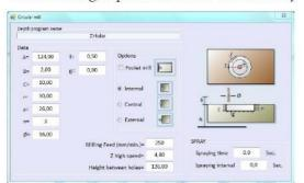
Circular milling with programmable finish-run
