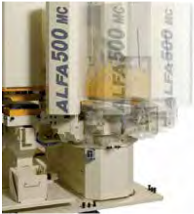
MITER SHEAR UNIT Flar bar cuts (-45 ° to +45 °)
