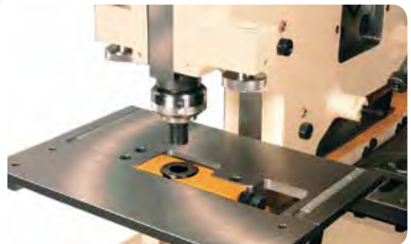
Goose neck die-holder for punching of L and I sections on legs and webs. Quick tool change.
