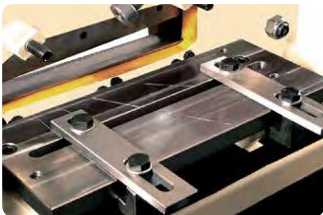
Anti-torsion system for flat bar shearing without deformation
