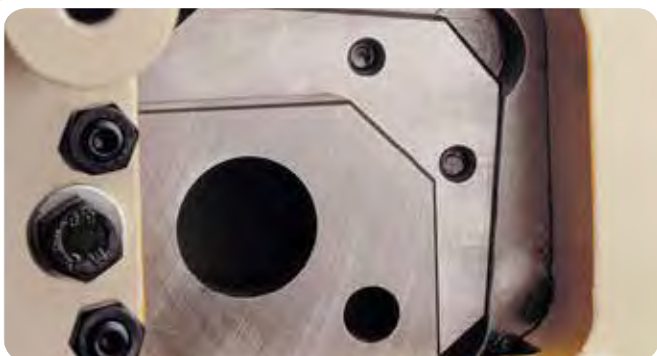
Blades for Øcut minimum deformation
