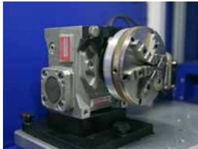
C axis to mark on cylindrical parts
