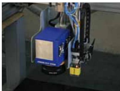
Integrated System for reading and verification of DataMatrix codes
