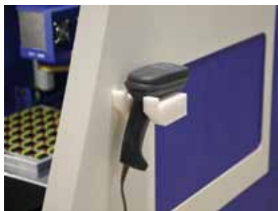
Selection of the program to be marked using a Bar Code Reader
