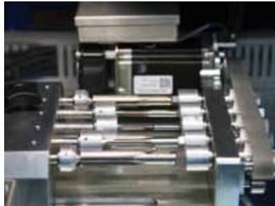
Multiple C axes (up to 10 spindles) with pneumatic operation
