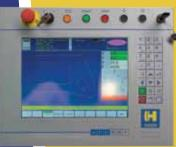
has a 15" TFT color display and comes standard with automatic cutting condition settings. Driven by high-performance, PC- based hardware, the APC59-T allows very fast processing of data and highly accurate calculation of plasma burning operations. The control has a high level plasma torch height control and communicates
