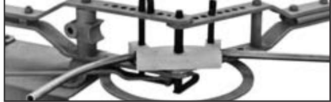
Feed-Along OD Tube Die Set (Form Die, Back Block, Draw Block) bending OD Tube to a large radius
