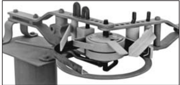
102B Form Die with attached Hold-Down Arms bending wide U-bend in Angle Iron, “Leg-In”, to a 2-3/4" radius
