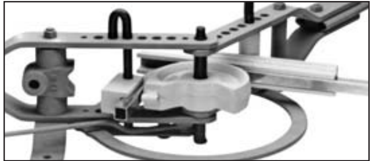
103B Square Tube 180° Die Set (Form Die, Back Block, Draw Block) bending a 4" radius in 3/4" Square Tube
