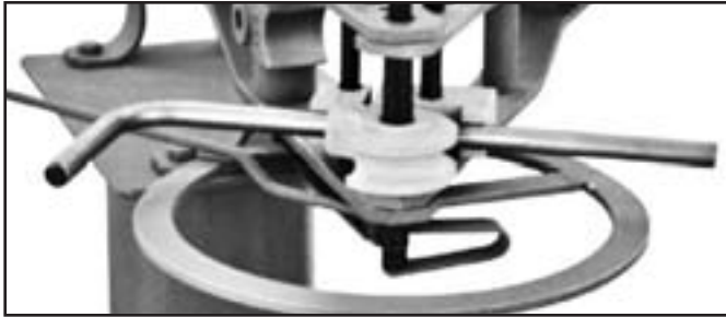
180° Pipe Die Set (Form Die, Back Block, Draw Block) bending Pipe to a short radius
