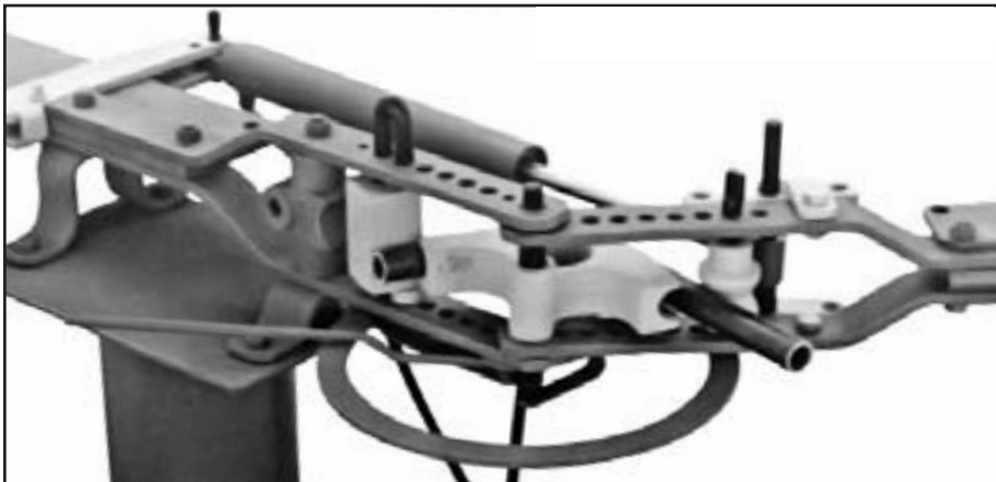
Hydraulic Cylinder attached using H55 90° "One-Stroke" Hydraulic Cylinder Mount. 44B Rigid Conduit 90° Die shown bending 1" Pipe to 90° with a single stroke
