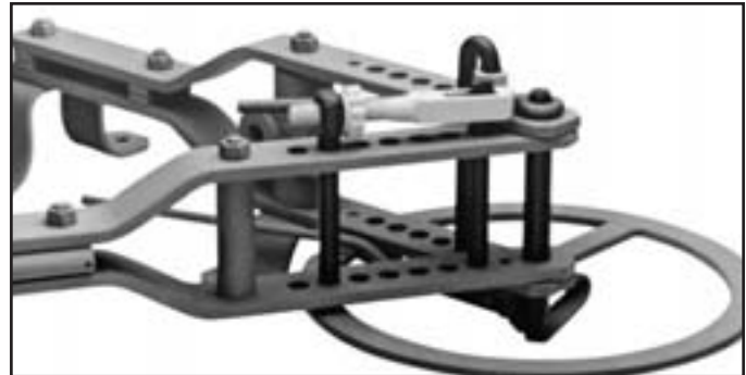
16B Eye-Bolt Bending Dog, toe to front, bending small-diameter Eye Bolt around 20B Center Pin on top of bender
