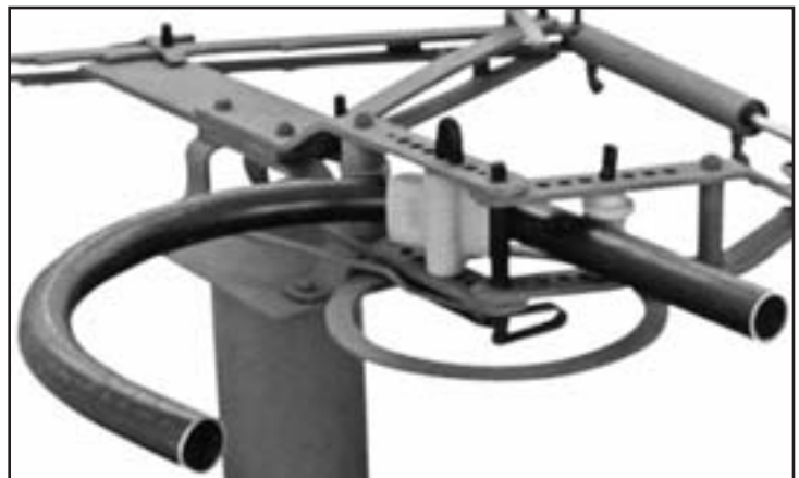
13B4 Pipe Die & 13B5 Roller bending 2" Pipe with hydraulic assist
