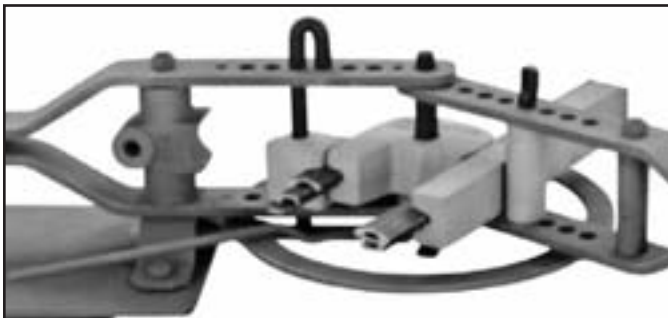
108B Die Set (Form Die, Back Block, long Draw Block) bending 3" radius in Handrail Cap and Structural Channel combined. Hydraulic Power recommended (not shown)
