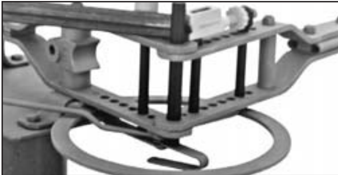
Bending tip of Lambs Tongue with 16B2 Wide-Nose Bending Dog
