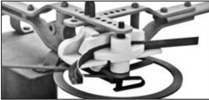
50B Master Die, 51B Outer Radius Block, 52B Inner Radius Block bending Angle Iron, "Leg-Out" Radius Block and 152B Back Block
