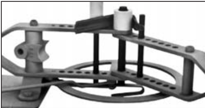
Completing Lambs Tongue using 20B7 Steel Roller
