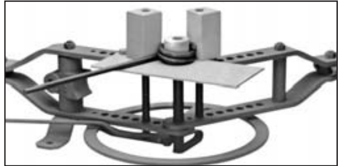
20B1 Round Cam mounted on 53B2 Center Pin and 20B2A Support Plate forms coil in Round Bar on top of the frame. 11B Square Blocks are used as backing blocks.
