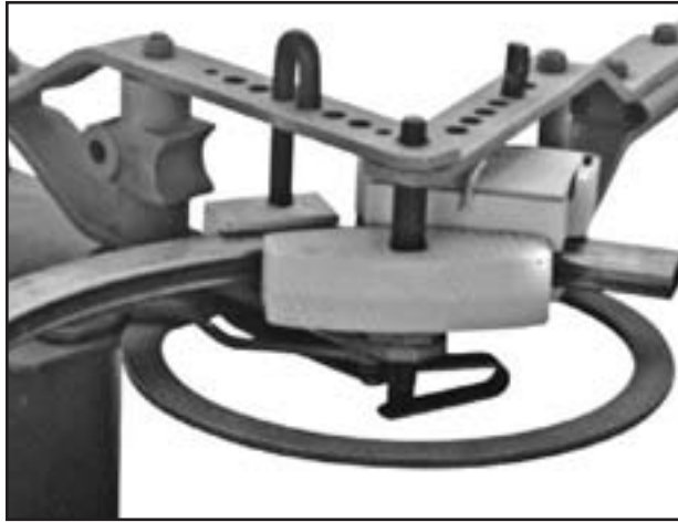
150B Master Die & 151B Inner Wedge grip stock as it bends along 154B "Crowned" Radius Block and 152B Back Block
