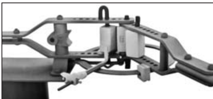
8B Cam Die (2") and 11B Square Blocks bend 'U'-Bolt in Round Stock to a predetermined point set by the 27B Circle Stop Gauge
