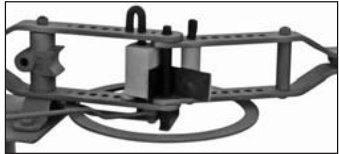
11B Block and 9B Roller bending 1/4" x 2-1/2" Flat Stock to a right angle
