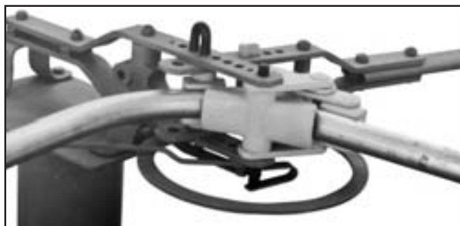
75B Feed-Along Form Die with Compound Linkage bending 2" Electrical Metallic Conduit
