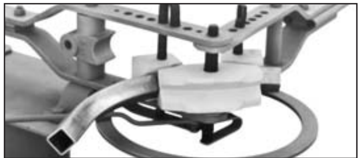
20B9 Form Die and Back Block/Draw Block Set bending Square Tube to a larger radius on the section diagonal
