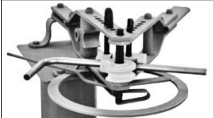
180° OD Tube Die Set (Form Die, Back Block, Draw Block) bending OD Tube to a small radius
