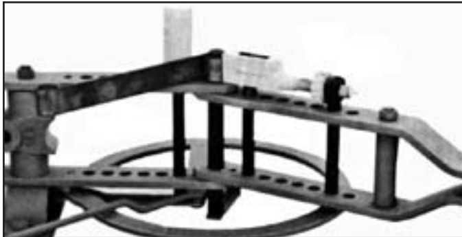
16B2 "Wide-Nose" Eye Bolt Bending Dog with longer 20B6 Long-End Center Pin and longer 53B1 Backing Pin & 9B Roller bending Eye in 1-1/2" x 1/8" Flat Stock
