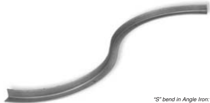
“S” bend in Angle Iron: “Leg-In” (top) and “Leg-Out” (bottom)
