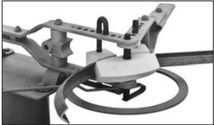
20B10 Form Die with 42990 Back Block/Draw Block Set bending Angle Iron with the “Heel Out”
