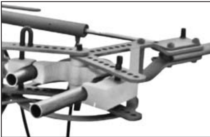
"L-Type" Swinging Frame bends 2" Pipe a full 180° using a 180° wrap-around-type die
