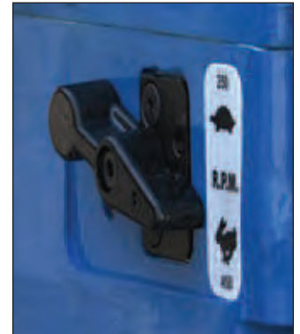
Two speed gear box for increased tool life
