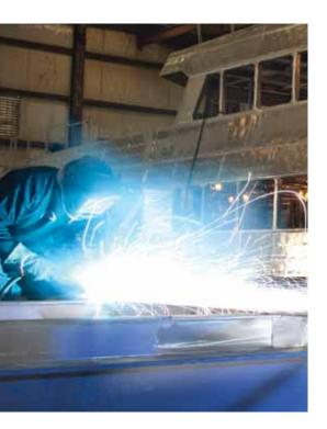
Plasma cuts any electrically-conductive metal, even painted or rusty metal, up to 4 times faster than oxyfuel.
