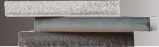
Relative cut performance on 12 mm (1/2”) mild steel
