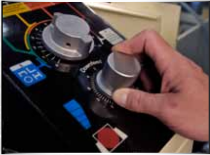
Bow Down-feed rate sets the cutting advance rate
