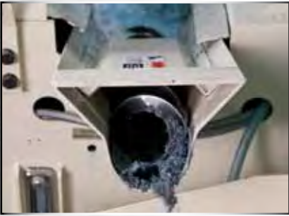
Automatic chip cleaning system
