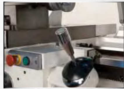
Joy stick design on the rapid power traverse on the cross slide and carriage makes it easier to use and comfortable in your hand.
