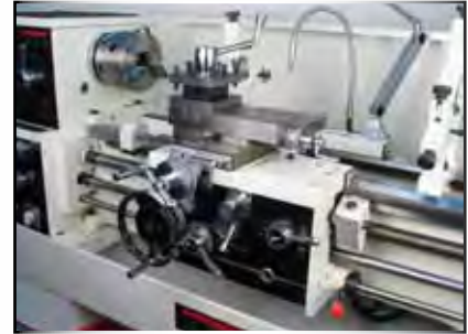
Carriage features One-shot lubrication and Turcite B on slide surfaces
