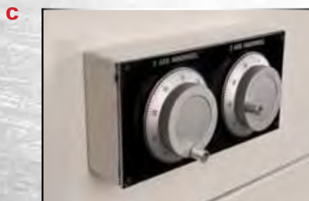
Electronic handwheels for initial positioning of tool.
