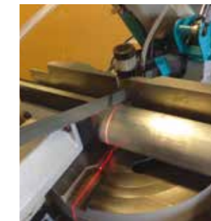
Laser line- Can be added to any bandsaw H310 and larger
