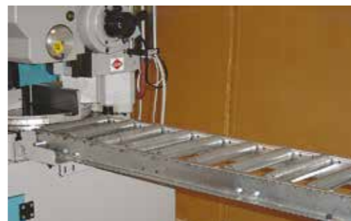
Custom machine mounted conveyors w/ micro adjustable legs. Available in 5' and 10' sections.
