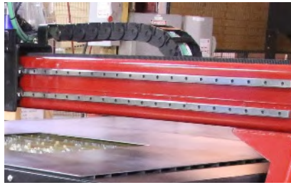
Heavy-duty Linear Bearings both "X" & "Y" Axis Provide smooth and accurate motion
