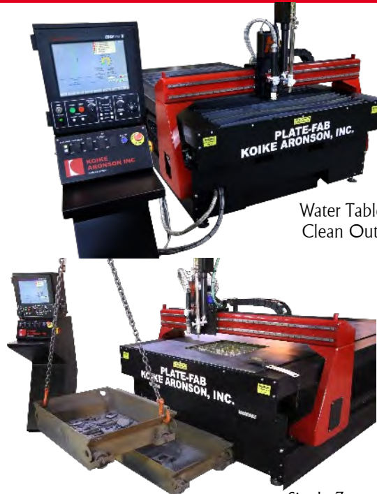
Single Zone Downdraft Table with roll out slag pans Optional: Fume extraction unit
