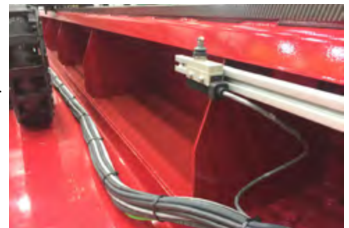
Main Beam Construction Solid steel fabricated construction. Includes precision machining for linear bearings and rack.
