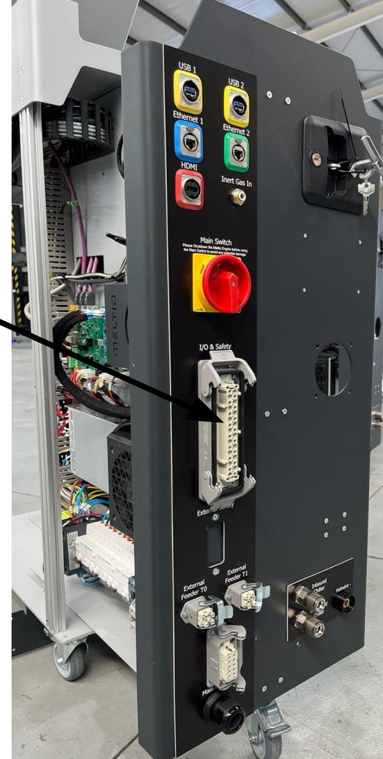
**Pins 1 to 16:** I/O communication (32p harting pinout attached).
