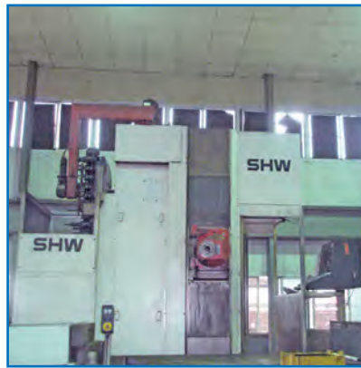
SHW 5-face boring
