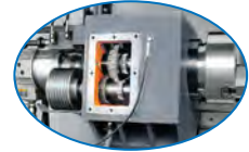
VT-27G has 2-step gear spindle
