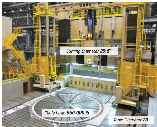
HTM - 7.0/9.0 GTN Gantry style 4-axis turning center.
