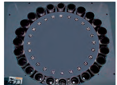
Lateral design prevents cutting fluid from flushing into tool pot.
