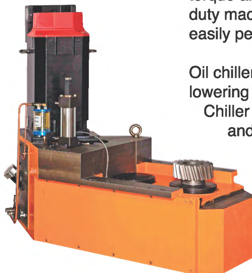
Gearbox slides in-and-out for easy maintenance
