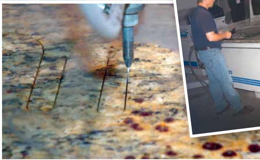
WaterJet cuts 3/4" granite
