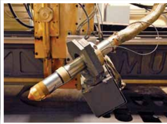
Optional Five-Axis Plasma head allows 3-D bevel cutting
