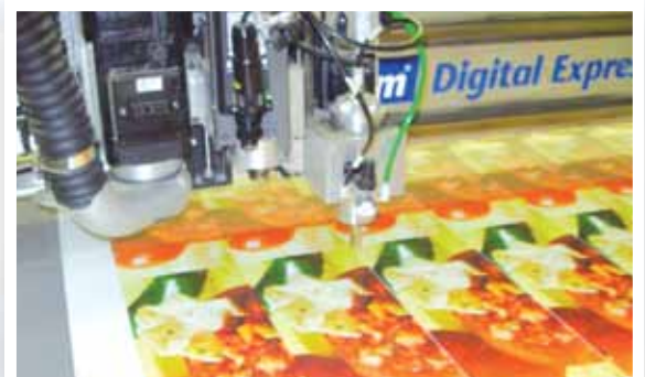
Featuring MultiVision digital registration, the Digital Express provides quick, accurate alignment.
