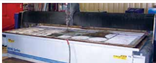
NTPV's MultiCam 3000 Series WaterJet features a 60" x 144" work surface.
