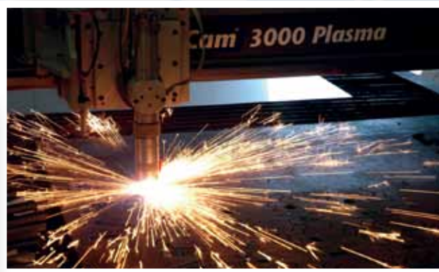
Cutting 1/2" plate steel with the 3000 Series Plasma and HPR 130
