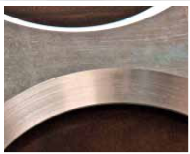
Beveled-aluminum part cut at high speed on 7000 Series Router
