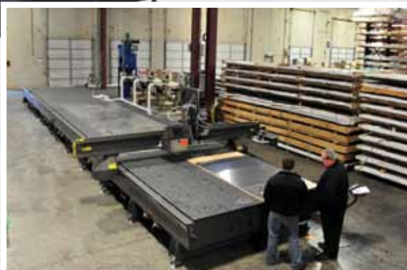
Custom 5000 Series Router has an 8' x 50' capacity
