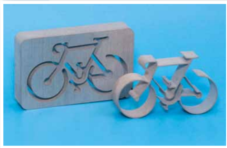
WaterJet-cut precision aluminum part
