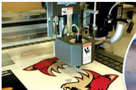
1000 Series Digital Finishing System with MultiVision, EZ Knife and 4-hp router
