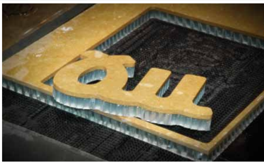
Architectural fascia cut on 3000 Series WaterJet
