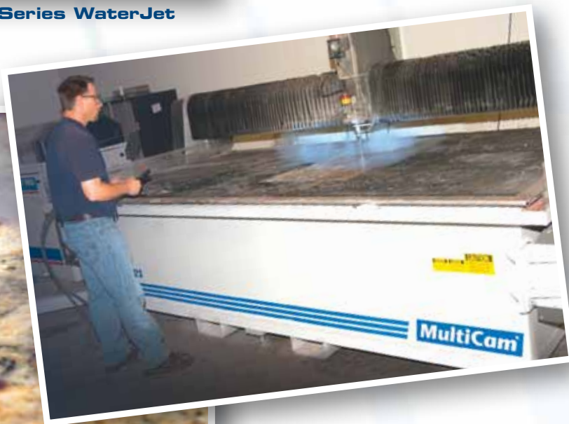
Architectural fascia cut on 3000 Series WaterJet
