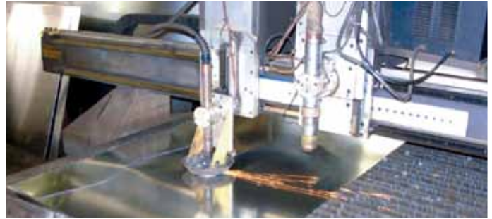
The MultiCam Plasma produces a clean, smooth, dross-free cut.
