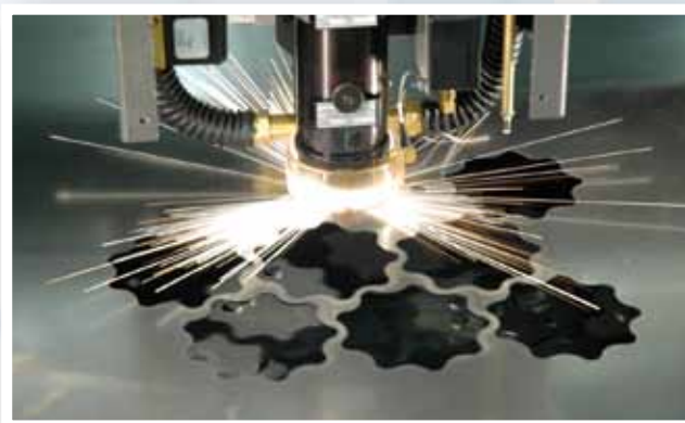
400-watt 2000 Series Laser cutting gauge steel
