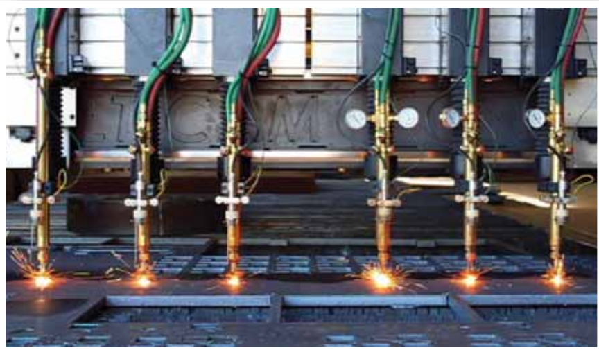
6000 Series Plasma with six-head oxy-fuel system
