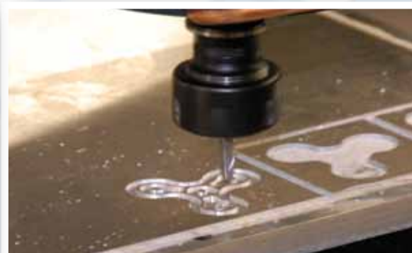
3000 Series Router cuts small aluminum parts
