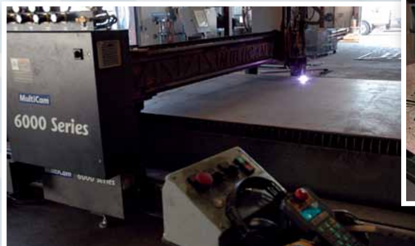
6000 Series Plasma with HPR 260 cuts 5/8" plate steel
