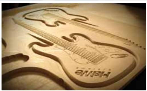
3-D carving of 3/4" MDF with 3000 Series Router
