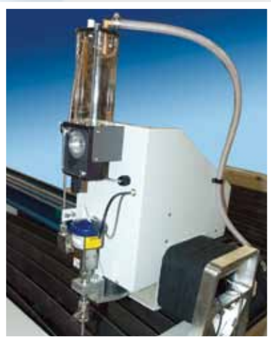
MultiFeeder abrasive feeder/bulk hopper system operates under full CNC program control
