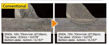
Bead with wide leg length and reduced throat thickness
