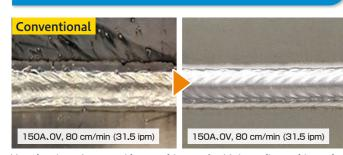
Very low heat input and less weld smut for high-quality weld results.
