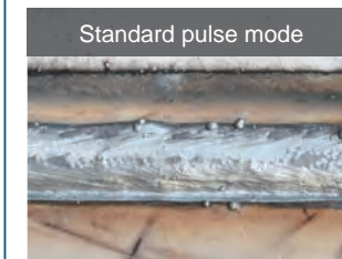
Spatter adhesion and undercut occur
