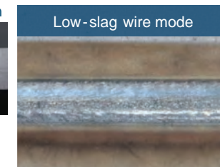
Good weld bead with no defects
