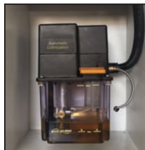
Fully integrated lubrication system
