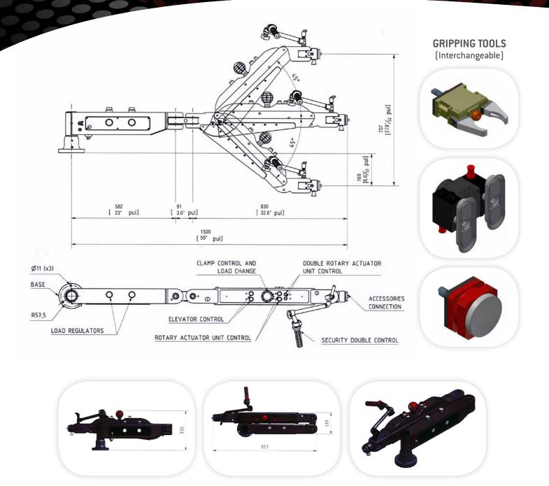
Features: Weight to handle: from 0 up to 25 kg. Radius working area 1.500 mm (+ usable), Vertical stroke 700 mm. Pneumatic equipment: Air Filter, 2 Precision regulator, Selector valve 2 preasures (2 loads), Security valve, Dual actuation system. Supply: Compressed air 7 bar. Base accessories: High base, Trolley and column, Tables, Lifters, Beam and Rails ( top, bottom and slide wall mounted), etc. Gripping Tools: Rotary actuator unit, Double actuator unit , Clamp, Vacuum, Magnetic, others
