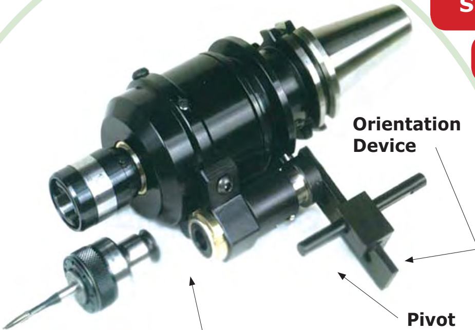
Grease Insertion Plug Add Grease Every 40,000 Threads
