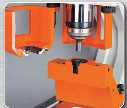
*Goose-neck die holder for punching channel flanges and webs.
