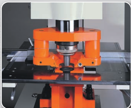
*Urethane spring stripper for minimal deformation.
