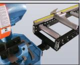
Roller Conveyor Available for Quick-Loc & Multi-Loc.
