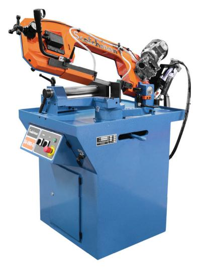
For larger material that requires a band saw, this scaled-down but rugged horizontal band saw can easily cut through round material up to 8" diameter, & features a swing head that can miter 60° right of 90°, giving you a 30° cut part without material movement.
