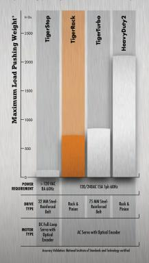
**TigerStop:** handles loads up to 120 pounds\*, an ideal and cost effective solution for non ferrous metals and lighter duty steel and ferrous metal applications.
