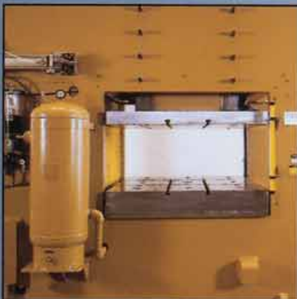
Typical window for model DCSS, shown with air tank for die cushion and an automatic lubrication system
