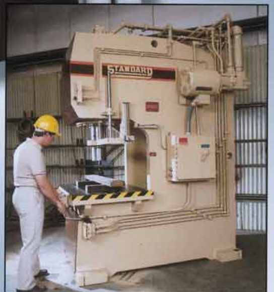
Special 200 ton C-frame style straightening press
