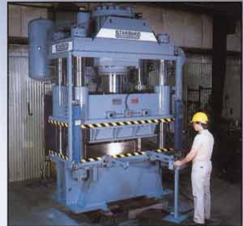
Model AP600 press with optional die bolster rollout arms; light curtain safety systems and air actuated quick change die system located in t-slots rubber pad box and paint color
