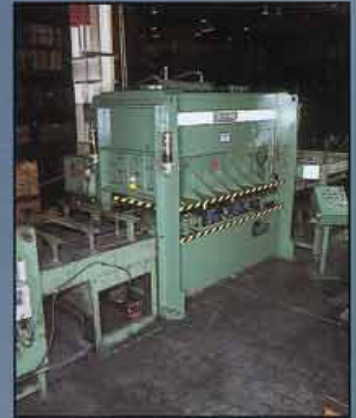
200 ton press in automated feed line & optional paint
