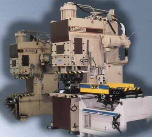
DC150 C-frame presses with optional PRE brand material feeding system
