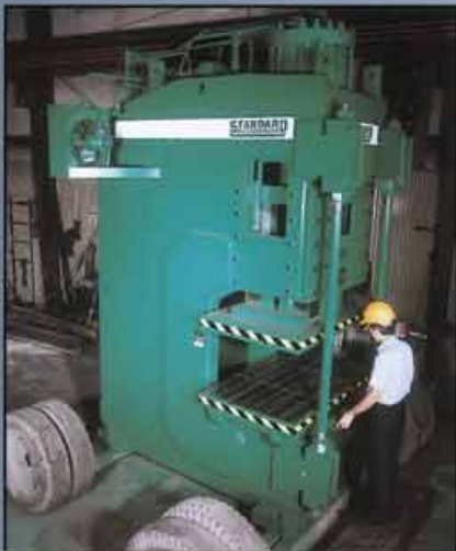
DC500 w/ optional support Tie rods and paint colors
