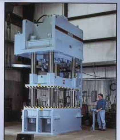
Model AP1000 with optional color (1,000 ton capacity)
