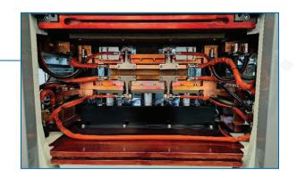
TECNA's patented perfect planarity improves the handling of large area multi point projection welding.
