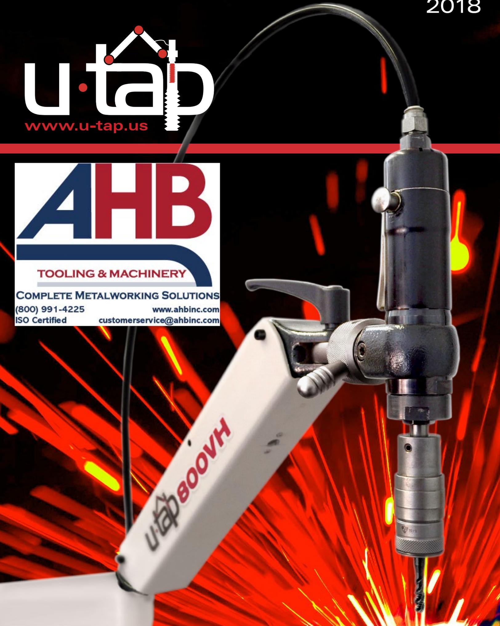
**The u-Tap Tapping Arm** consists of a radial arm connected to a tilting arm that is balanced by a pneumatic damper. The tilting arm fixes to the head member and pneumatic motor, and works in a perpendicular axis to the work piece. The u-Tap 400VH and 800VH additionally offer the ability to tap vertically or horizontally. The pneumatic motor is available in 2 speeds, 400 or 800 RPM.
