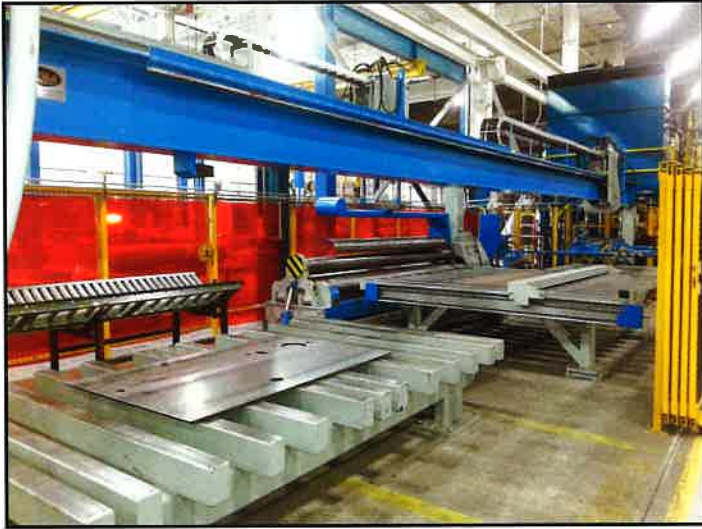
403-10-12 rolling cell for rolling natural gas tanks for vehicles
