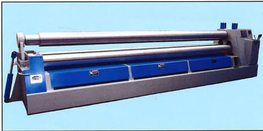
101-8-16 w/Polished Rolls, Manual Hydraulic Valves, & Long Length to Roll Architectural Components
