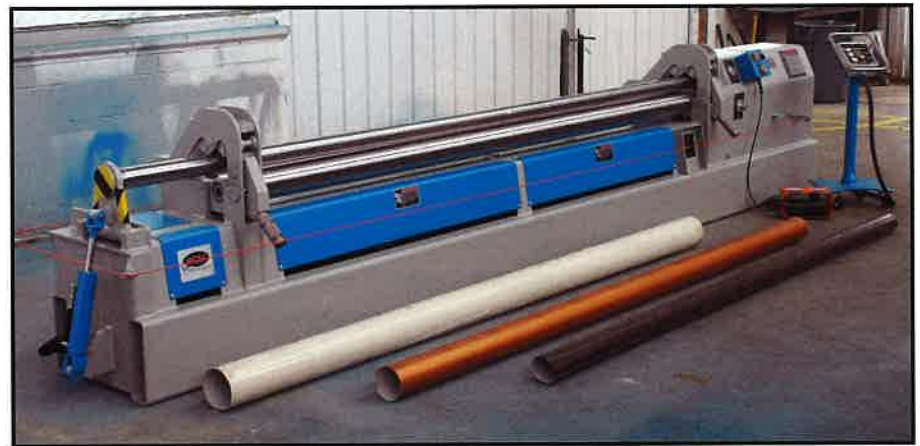
KRR-3.5-120 rigidified top roll initial pinch rolling gutter down spouts
