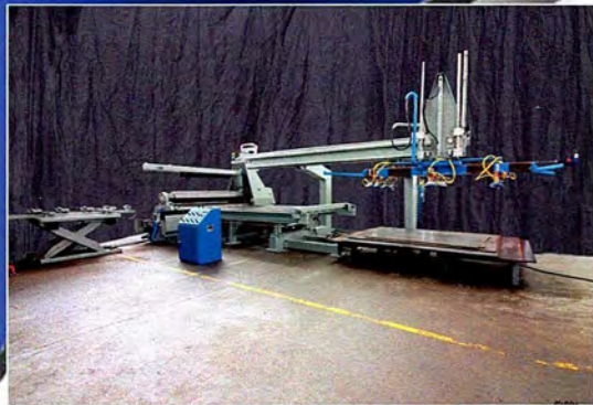
403-13-8 rolling cell to form propane tanks
