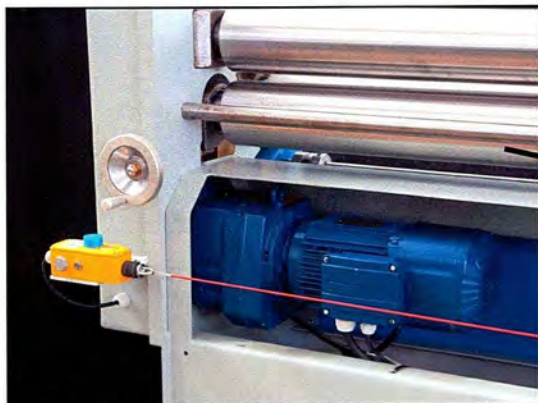
Safety cable switch. Helical gear motor with electric holding brake for roll drive. Total electric operation. Near instant start-stop-reverse. NEMA premium efficient motors. Gearbox lubed for life
