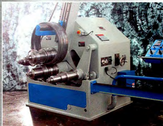
SRR-44 for rolling steel wheels for farm machinery
