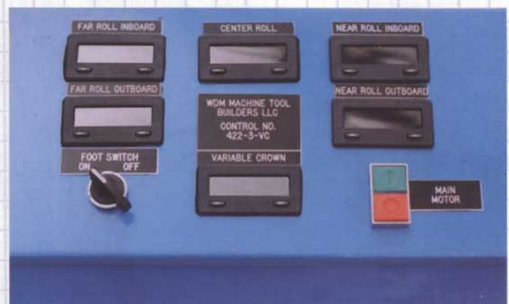
Variable crown position is indicated via electronic digital readout. See photograph above.
