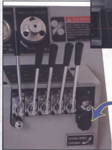
Close up view of system speed control knob on a manual control style.
