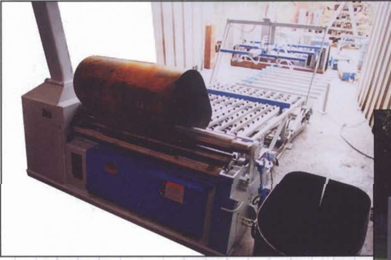
400-5-5 (.135" x 5') with automatic feeder rolling D-shaped automotive fuel tanks automatically.
