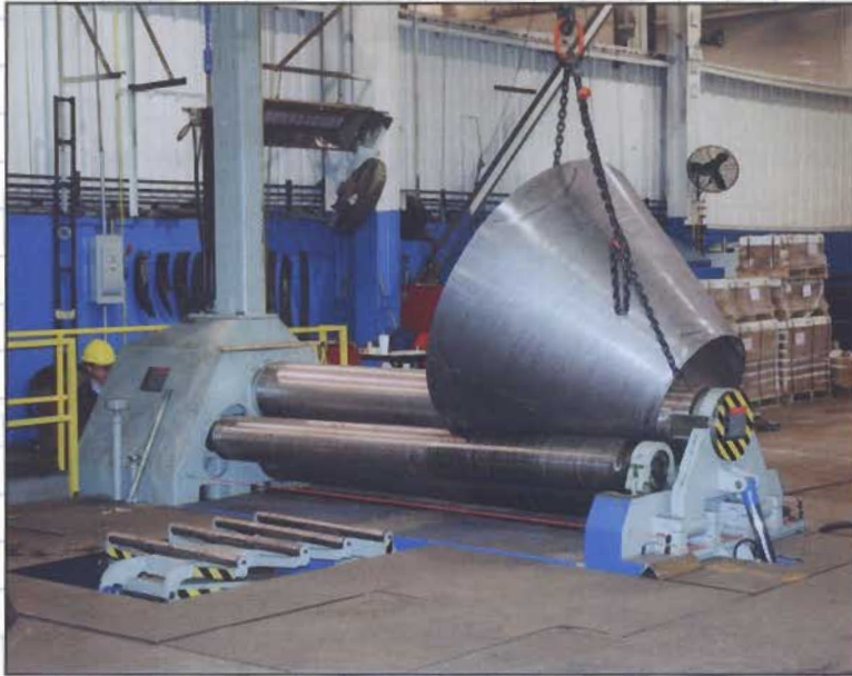
403-16-10 (57/64" x 10') with side and overhead supports used to manufacture silos and related parts for asphalt production.
