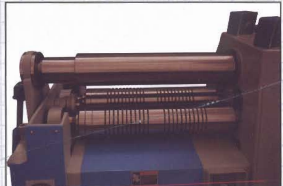
Special three roll pinch pyramid with grooves for forming fan housings.
