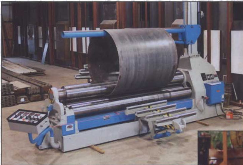
403-12-10 (1/2" x 10') with side and overhead supports, swinging console control and 423-LP-6 control used for process and dust collection equipment.
