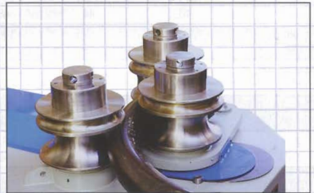
Pipe dies on PPSR-61 Section Roll (no guide rolls) rolling a large pipe section.
