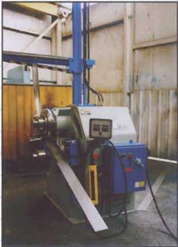
AR-40 with overhead support forming stainless steel half pipes in one pass.
