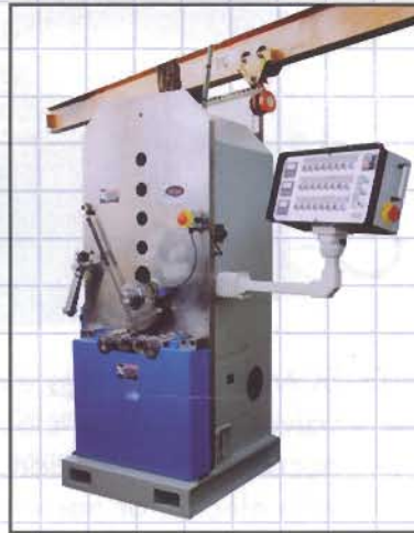
Specially designed and built machine to form orthopedic components for hip replacements.
