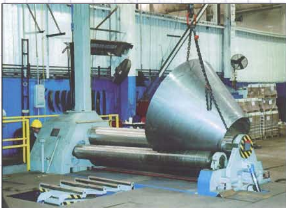
3/4 x 10 Four Roll plate bending machine with side and overhead supports.
