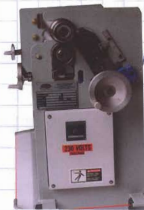
Drop end view of B machine shows location of electrical box, pinch roll adjusting hand wheel, and position scale. Notice the alloy steel bearing case and wedge screw arrangement for accurate positioning of the pinch roll.
