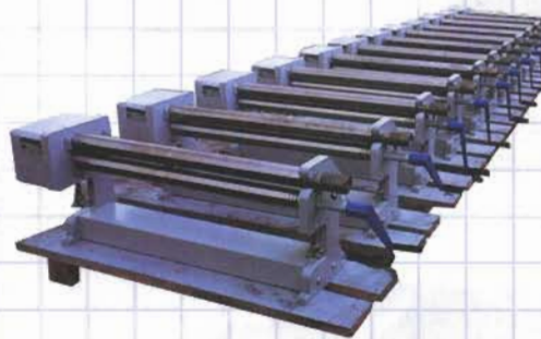
Group of 2.5-36 manual sheet rolls used in maintenance shops and sheet metal trades.
