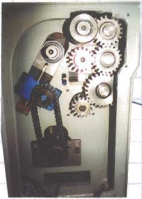
Heavy duty all gear drive for rolls. Roller chain drive for power bending adjustment.
