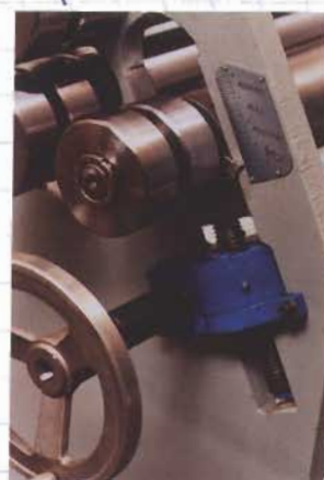
Shows standard scale pointer which shows the position of the bending roll.
