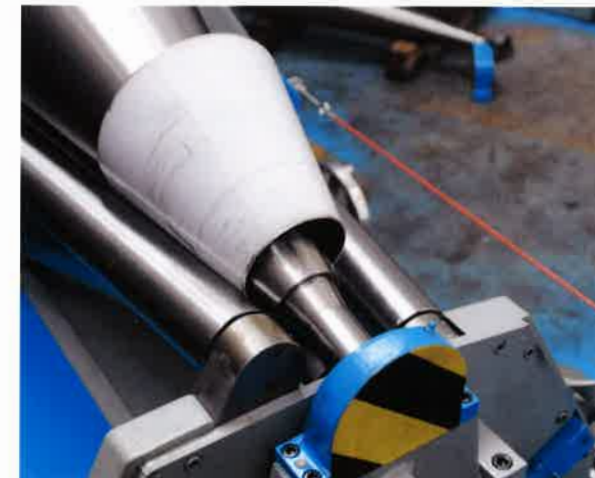
Rolls rotate to complete the forming cycle in 1 pass without any twist or edge deformation from a cone snubber (as with traditional rolls).
