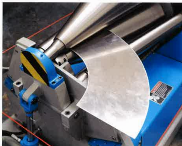
Work piece is entered into the machine & positioned via the calibrated pointer & gage roll.
