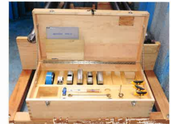
Tool chest open showing extra bearing holders & changing tools
