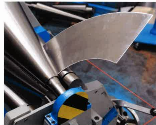
Near forming roll is raised to form leading edge. Rolls rotate to complete bend.
