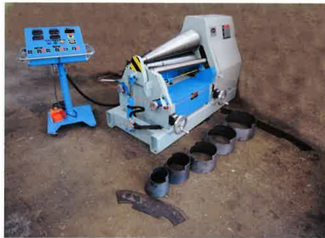
Asymmetrical cones for grain handling
