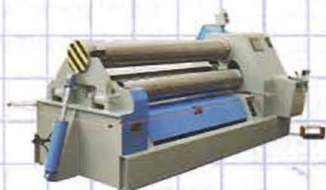
101-10-8 (1/2" x 8') hydraulic pinch pyramid plate bending machine.
