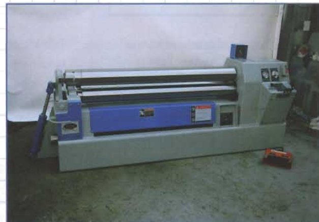
K-6-6 (1/4" x 6') with optional cone attachment and roll rotation foot pedal.
