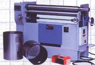
B-3-5-36 (12 gauge x 3') sheet metal roll
