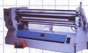
B-6-72 (7/32" x 6') with rod grooves. This machine is an economical alternative to the K series machine.
