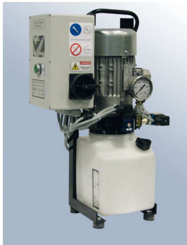
Hydraulic Power Pack HM10 and HM11 type H (Manual operation) or C (linked to the CNC control).
