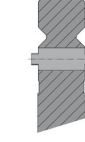
HD Safety-Pin Applicable for tool weight > 12.5 kg/28 lbs - < 150 kg/331 lbs. (NS I + II)
