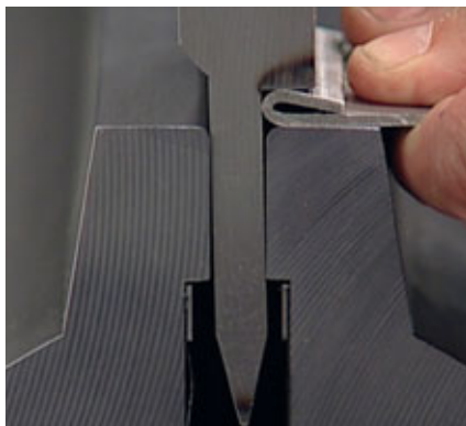
Pre-bend and flattening in the same tool.
