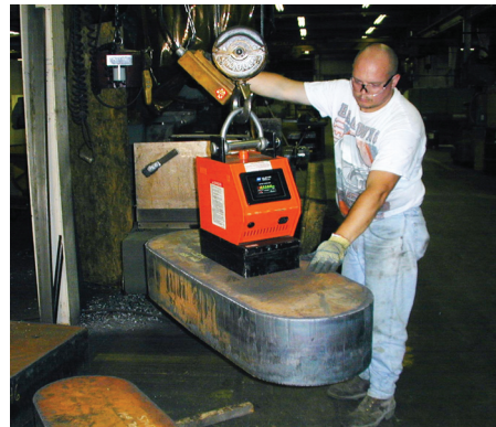
Infra-Red Remote Control Walker Self-Contained Battery Lift Magnets can lift steel up to 11,000 lbs.
