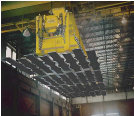
Flame cut parts can be lifted all at one time
