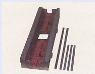
Hardend and ground ways with turcite on opposing surfaces and gibs.
