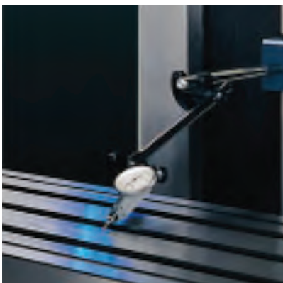
Parallelism of Table Surface to Ram Cross Transverse Movement Less than 0.0008" per 12" of travel
