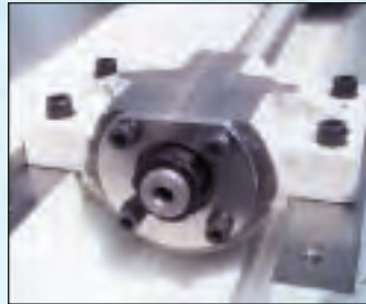
Precision ballscrews supported at both ends.
