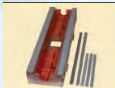
Hardened and ground ways with Turcite on opposing surfaces and gibs.
