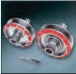
Dynamically balanced pulley with special bronze key attached with 2 screws prevents premature breakage.
