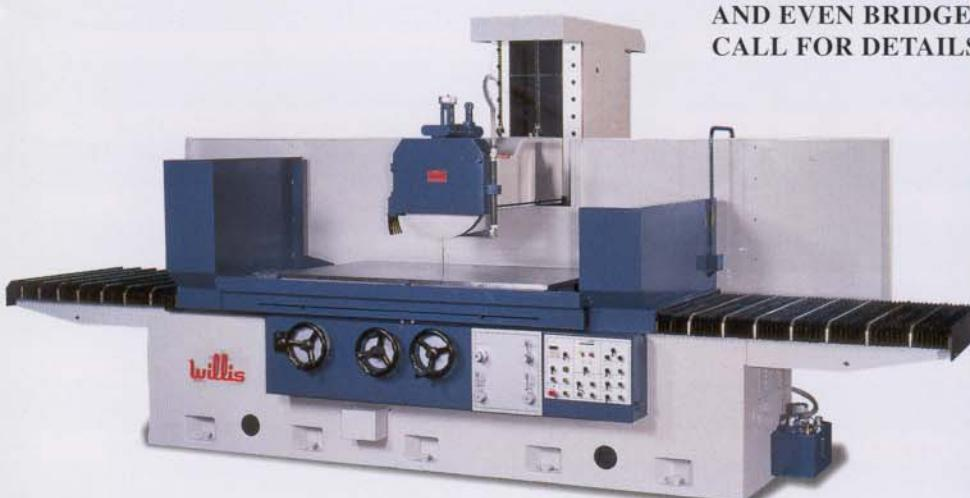
32x"80" table working area, 34.2" x 88.6" maximum travels, 15HP spindle motor, V and flat turcite ways for table feed, traveling column for crossfeed, hydraulic table feed, hydraulic incremental crossfeed, automatic incremental downfeed, automatic lubrication rear splashguard, PLC control crossfeed traverse, (2) 32x40 electromagnetic chucks and control, magnetic separator paper filter coolant system, hydraulic dresser.
