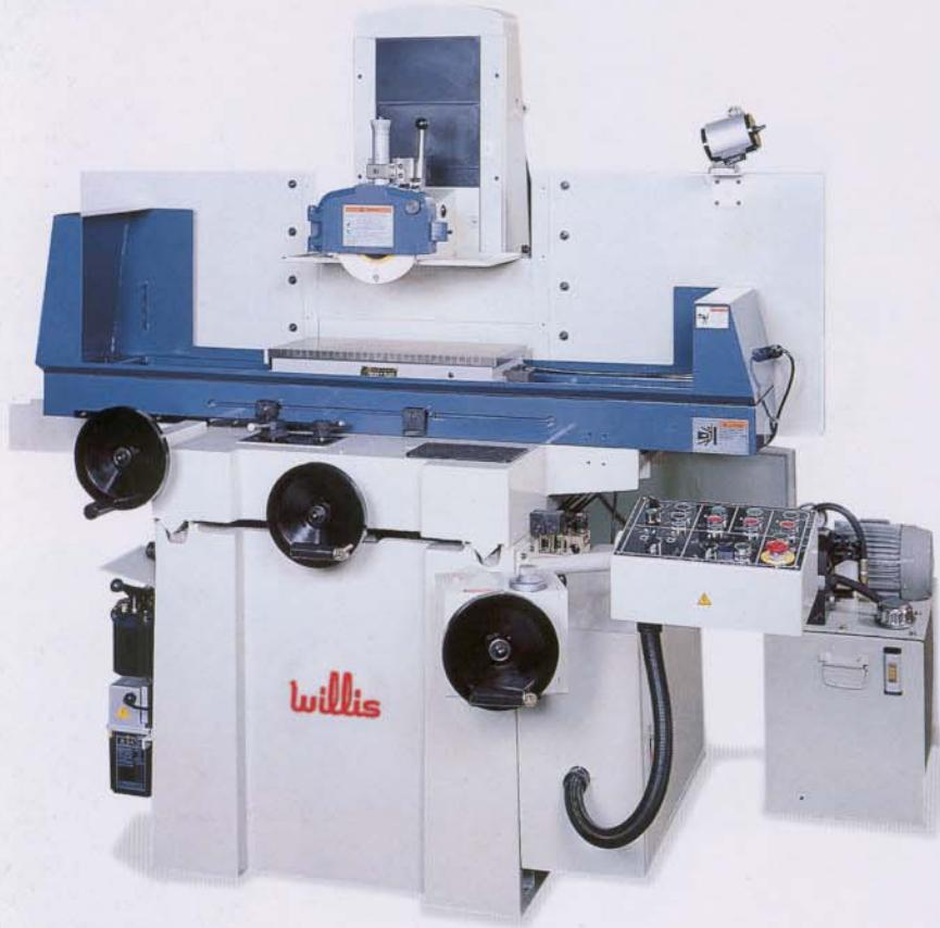
10"x20" table working area, 10.8"x21.0" maximum travels, 3HP spindle motor, V and flat turcite ways for table feed, hydraulic table feed, electronic control crossfeed, automatic incremental downfeed, automatic lubrication, rear splash-guard, 10x20 permanent chuck, dust suction and coolant system, parallel dresser.
