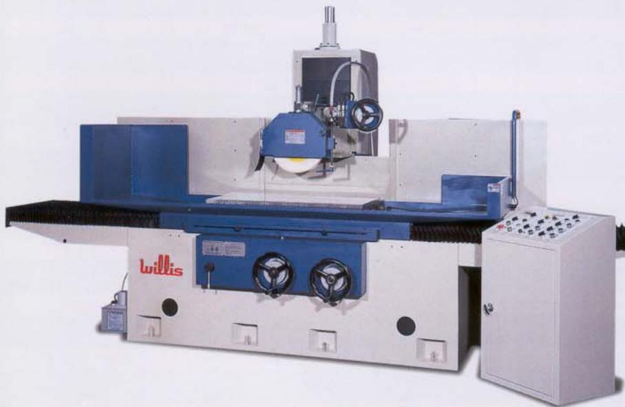
20" x 40" table working area, 22.5" x 45" maximum travels, 10HP spindle motor, V and flat turcite ways for table feed, traveling column for crossfeed, hydraulic table feed, electronic control crossfeed, automatic incremental downfeed, automatic lubrication, rear splashguard, 20 x 40 electromagnetic chuck and control, paper filter coolant system, parallel dresser.
