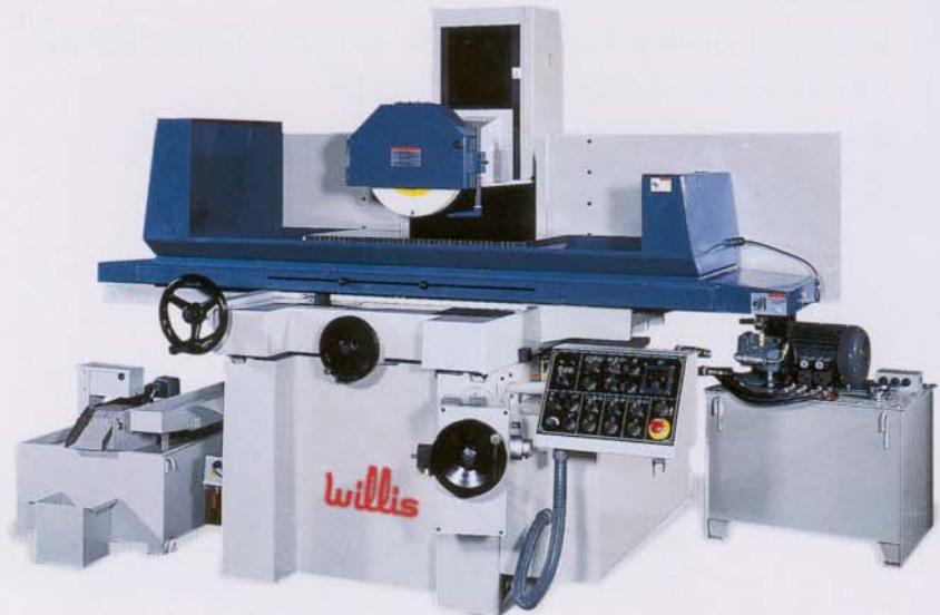
16" x 32" table working area, 17.7" x 36.6" maximum travels, 7.5HP spindle motor, V and flat turcite ways for table feed, hydraulic table feed, electronic control crossfeed, automatic incremental downfeed, automatic lubrication, rear splashguard, 16x32 electromagnetic chuck and control, paper filter coolant system, parallel dresser.
