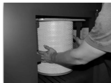
3. Slide filter cartridge(s) out
