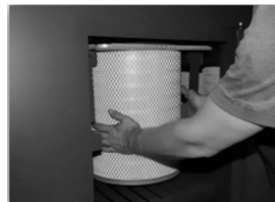
6. Insert clean replacement filter.
