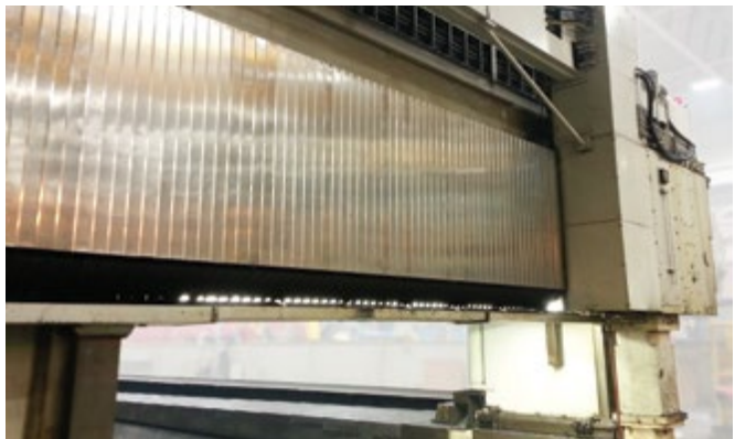
Gordillo bellows covers for machine way protection. Gordillo covers have been successfully applied in vertical, horizontal and crossrail configurations.
