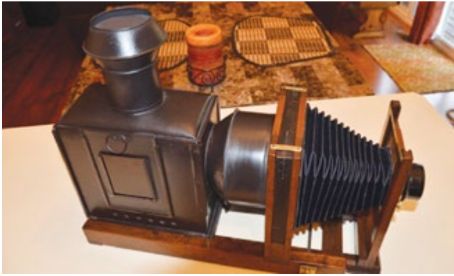
Light-tight folded Gortite® bellows used on a photo enlarger, folded construction.
