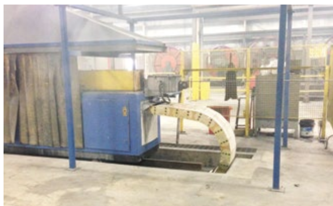
Enclosed-style Gortrac steel XL carrier in steel cable heat-treating application for unsupported long travel. Armor plates protect cables in aggressive environments.
