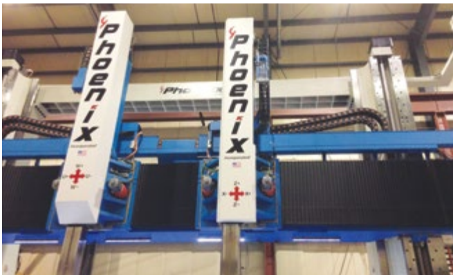
Gortite way covers and Nylatrac cable carriers on a large vertical machining center.
