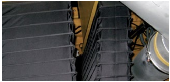
A Gorframe bellows provides flexible ducting on a large mining truck.
