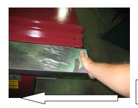
Push Rail toward the rear of the machine. This will drop the rail down.
