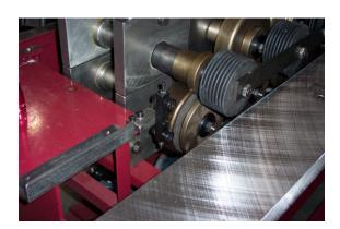
1. <u>Upward or downward bow:</u> This is controlled by the cams located on the exit end of the machine. If the form bows downward, adjust the 2 cams upward. If the form bows upward, adjust the 2 cams downward.
